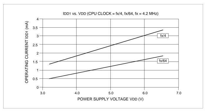
Figure 47. V<sub>DD</sub> VS. I<sub>DD1</sub>
