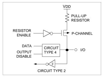
Figure 7. Pin Circuit Type 5
