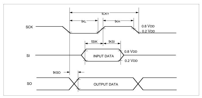
Figure 44. Serial Data Transfer Timing
