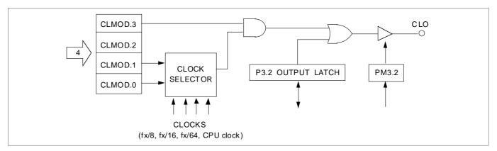
Figure 20. CLO Output Pin Circuit Diagram
