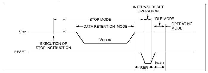
Figure 38. Stop Mode Release Timing When Initiated By RESET
