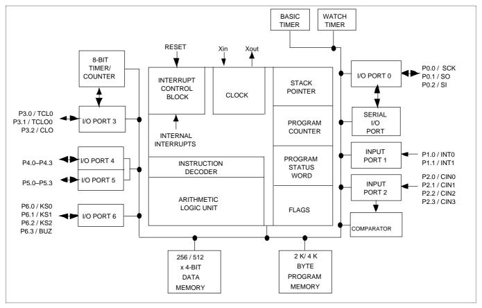
Figure 1. KS57C0002/0004 Block Diagram
