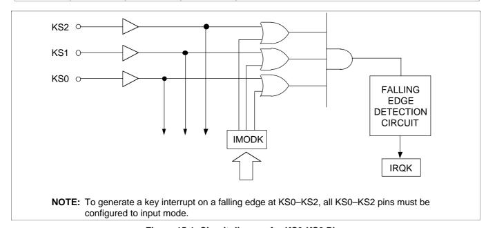
Figure 15-1. Circuit diagram for KS0-KS2 Pins
