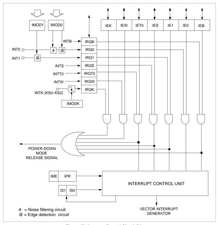
Figure 15. Interrupt Control Circuit Diagram
