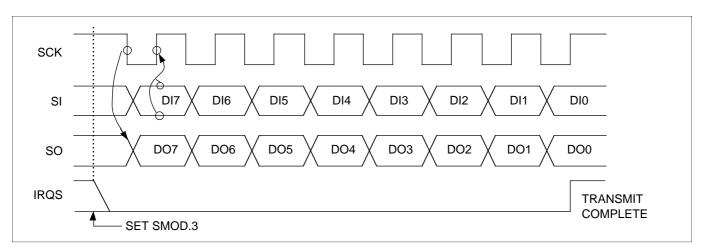
Figure 34. SIO Timing in Transmit/Receive Mode
