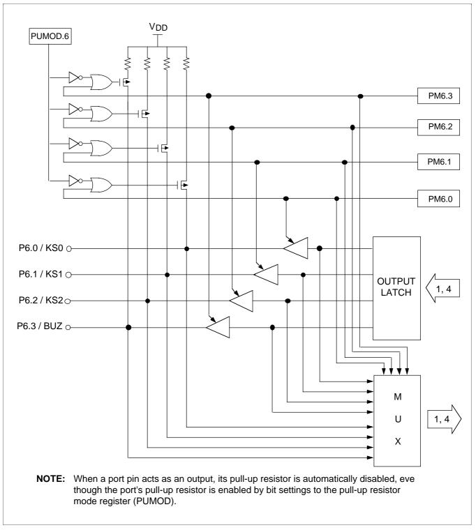
Figure 26. Port 6 Circuit Diagram
