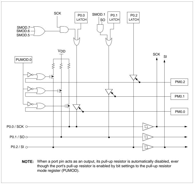
Figure 21. I/O Port 0 Circuit Diagram
