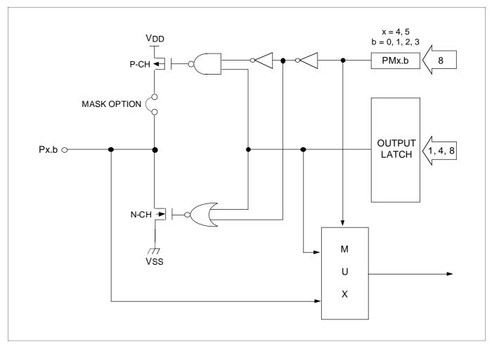
Figure 25. Circuit Diagram for Ports 4 and 5
