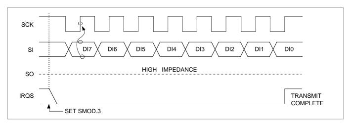
Figure 35. SIO Timing in Receive-Only Mode
