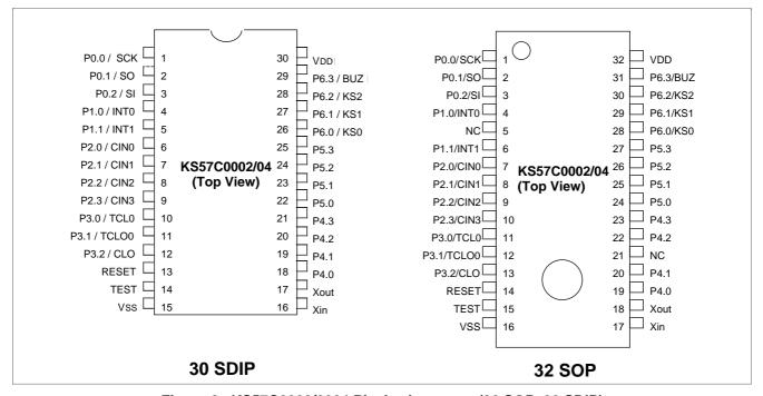
Figure 2. KS57C0002/0004 Pin Assignments (32 SOP, 30 SDIP)
