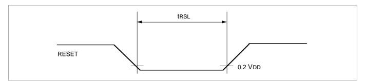
Figure 42. Input Timing for RESET Signal
