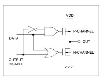
Figure 6. Pin Circuit Type 4
