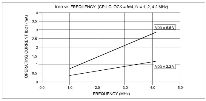
Figure 45. Frequency VS. I<sub>DD1</sub>
