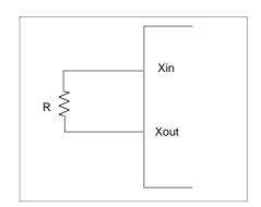
Figure 17. Crystal/Ceramic Oscillator
