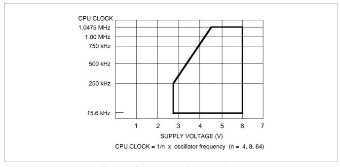
Figure 36. Standard Operating Voltage Range
