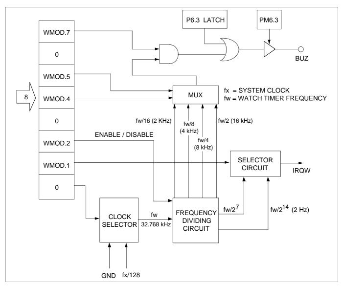
Figure 29. Watch Timer Circuit Diagram
