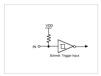
Figure 11. Pin Circuit Type 9
