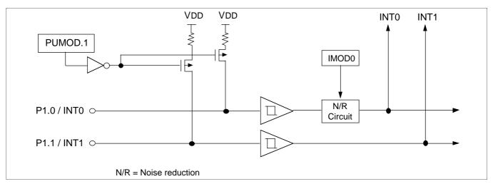
Figure 22. Input Port 1 Circuit Diagram
