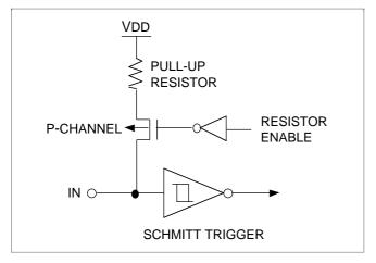
Figure 5. Pin Circuit Type 3
