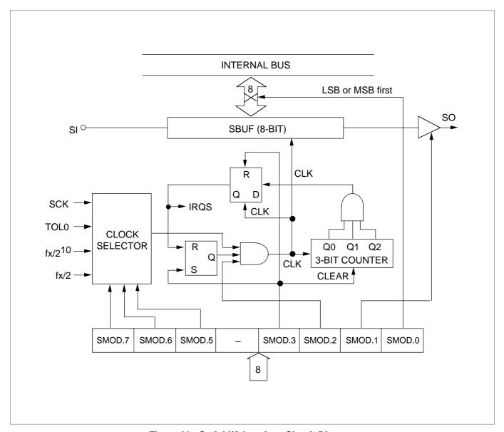
Figure 33. Serial I/O Interface Circuit Diagram
