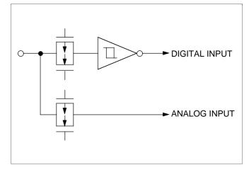
Figure 8. Pin Circuit Type 6
