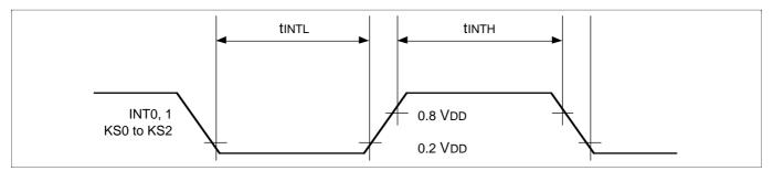
Figure 43. Input Timing for External Interrupts
