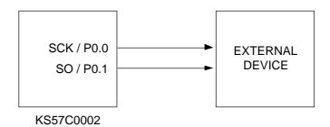
2. Use CPU clock to transfer and receive serial data at high speed:
