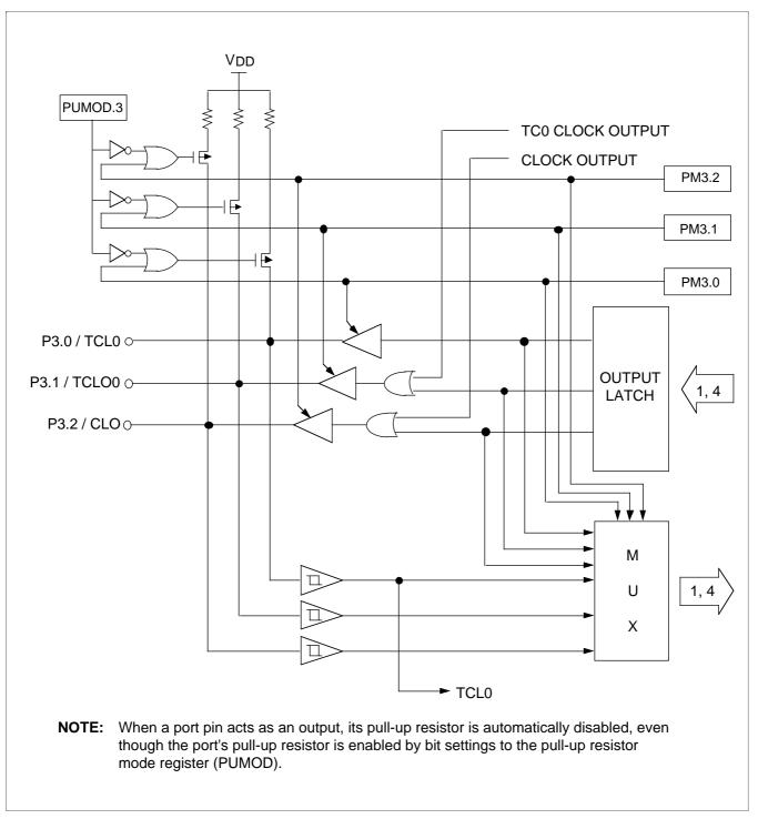
Figure 24. Port 3 Circuit Diagram
