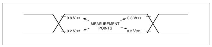
Figure 37. A.C. Timing Measurement Points (Except for Xin)
