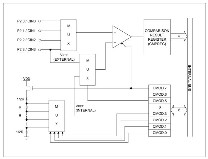
Figure 30 Comparator Circuit Diagram
