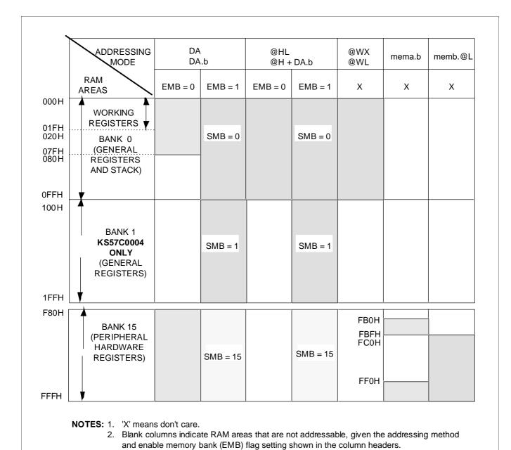
Figure 14. Data Memory (RAM) Address Structure
