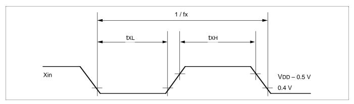
Figure 40 Clock Timing Measurement at Xin
